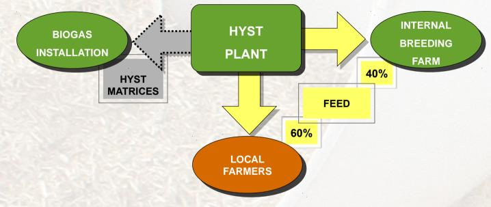
Processing the same biomass waste, the Hyst plant obtains feedstuffs for livestock and matrices for the production of biogas:
