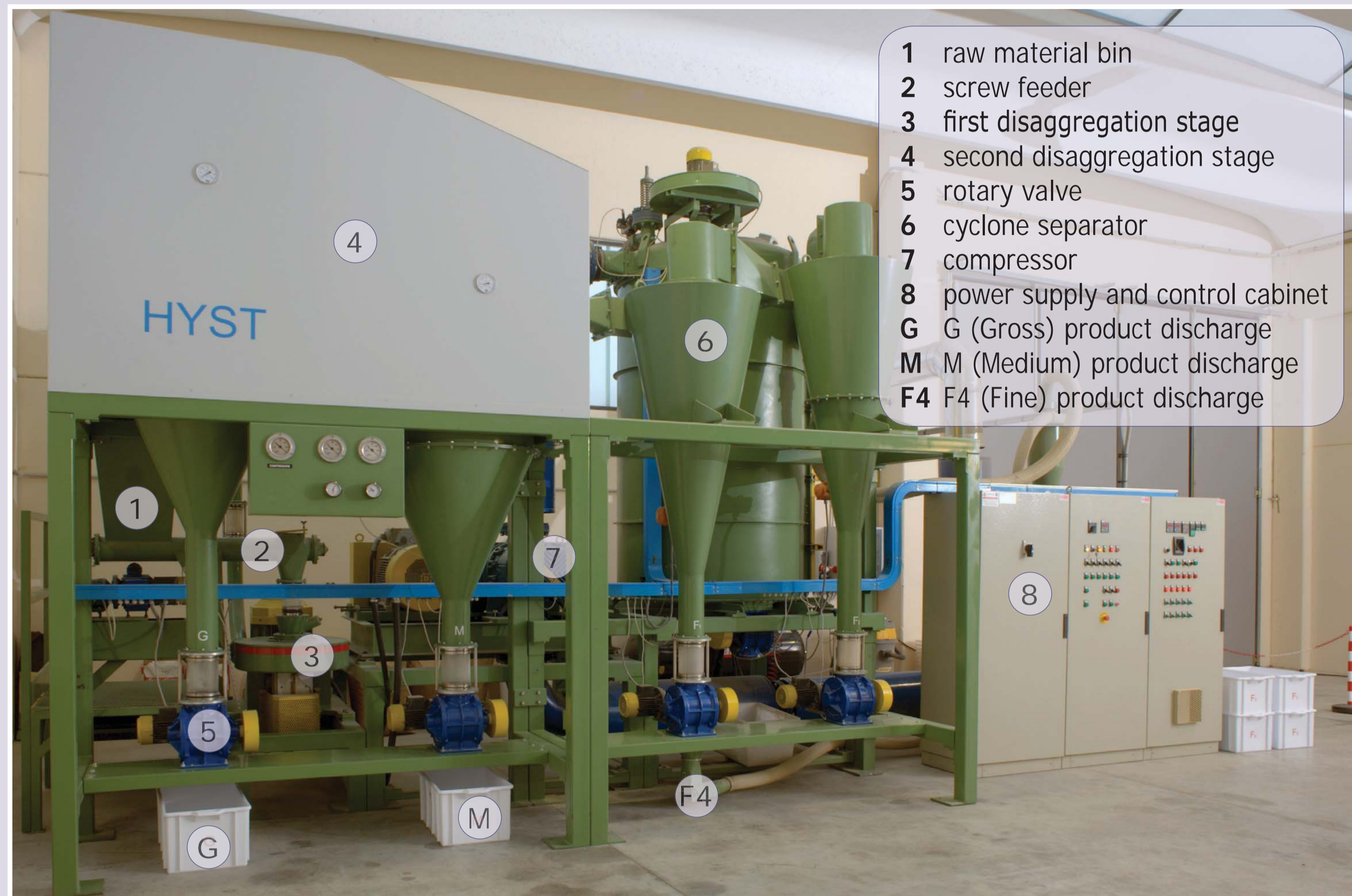
Figure 1: The HYST plant used to process wheat bran and corn stover
